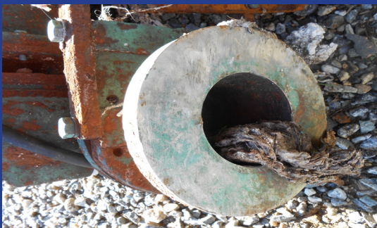
Taylor Pond sewage pump clogged with wet wipes
